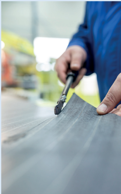
Karl Eugen Fischer manufactures machines that produce steel cord, the supporting structure of a tyre. So that the material can be cut cleanly, the cutting knife is heated.
